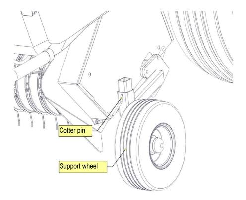
Figure 11. Adjusting working height of the pick-up
