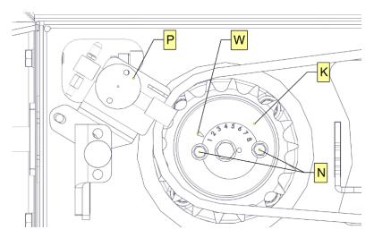
Figure 33. Adjusting the oil amount in the automatic lubrication system
