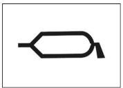
Figure 31. Marking of the main baler lubrication places
