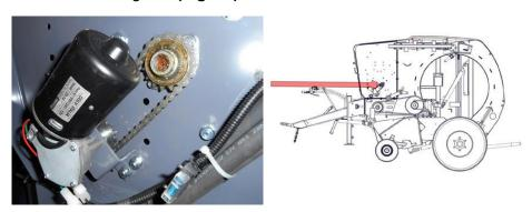
Figure 32. Lubricating the net chain
