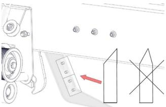
Figure 25. Sharpening the blade
