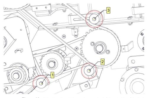
Figure 16. Adjusting the chain tension on the left-hand side of the baler
