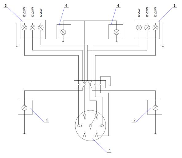
**Figure 37.** Electrical wiring diagram (1 – connection plug, 2 – head light, 3 – tail light, 4 – licence plate light)
