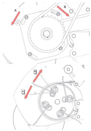
Figure 22. Pick-up cam adjustment
