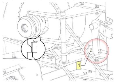
Figure 20. Adjusting the jaw coupling
