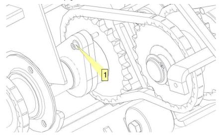
Figure 23. Replacing the locking bolt
