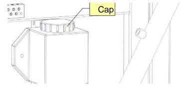
Figure 34. Oil tank of the automatic chain lubrication system
