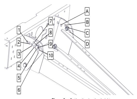
Figure 3. Setting the drawbar height
