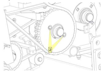
Figure 24. Replacing the locking bolt in the rolling roller protective device
