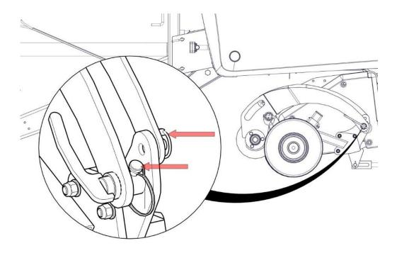
Figure 8. Wide windrow clamp dismantling
