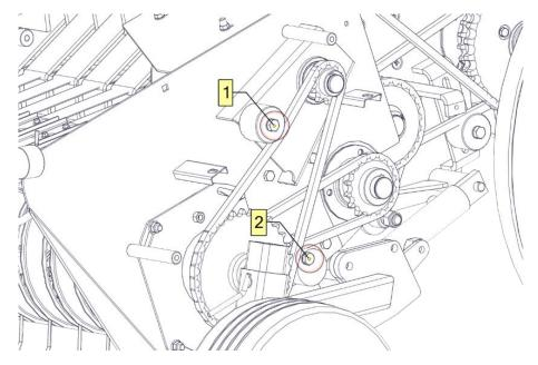
Figure 15. Adjusting the tension of the pick-up chains
