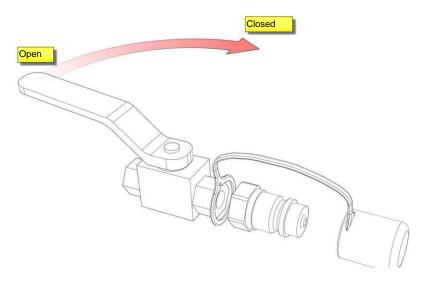
Figure 6. Cut-off valve
