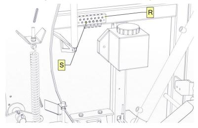
Figure 35. The bearing central lubrication system on the left-hand side of the baler
