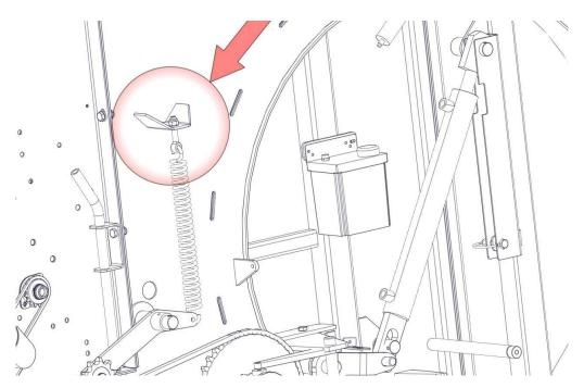
Figure 14. Adjusting the automatic chain tensioners
