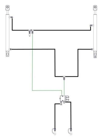
Figure 38. Diagram of the hydraulic system – rear chamber
