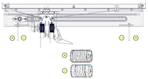
Figure 26. Binding width adjustment
