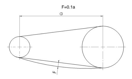
Figure 13. Chain tension
