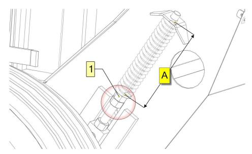
Figure 18. Adjusting the tension of the chain and rod conveyor set of the Z587 baler
