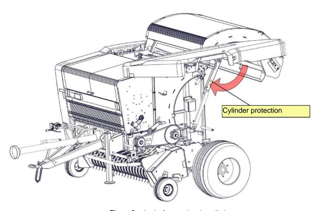
Figure 9. Locks for securing the cylinders
