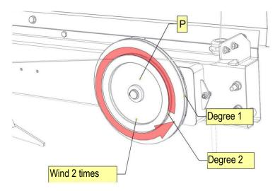
Figure 27. Twine bale binding density adjustment
