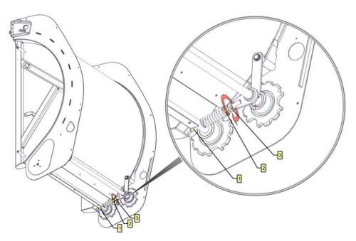
Figure 19. Adjusting the tension of the chain and rod conveyor set of the Z587/1 baler
