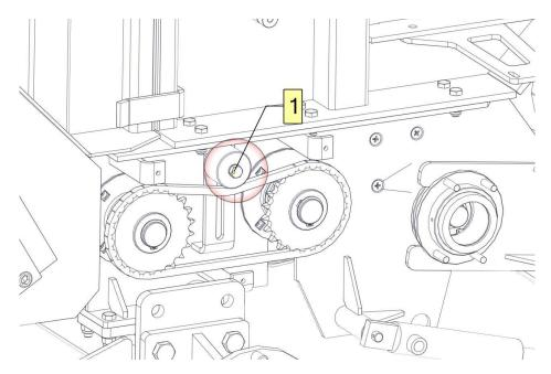
Figure 17. Adjusting the chain tension on the right-hand side of the baler
