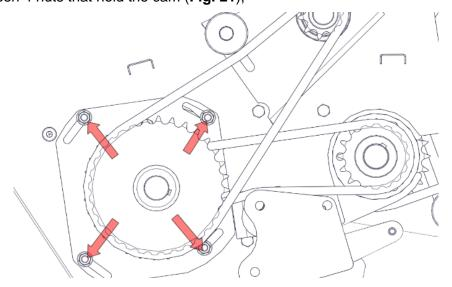
Figure 21. Pick-up cam adjustment
