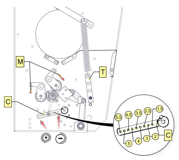
Figure 28. Net binding device adjustment
